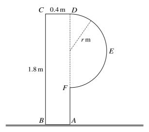
The diagram shows the cross-section ABCDEF through the centre of mass of a uniform prism which rests with AB on rough horizontal ground. ABCD is a rectangle with AB = CD = 0.4 m and BC = AD = 1.8 m. The other part of the cross-section is a semicircle with diameter DF and radius r m.
